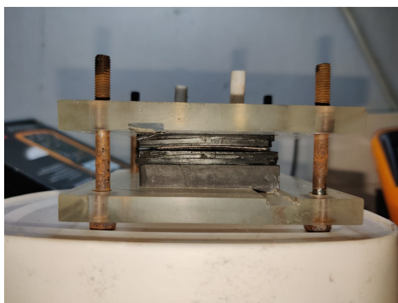
Figure 3.1: Zinc-bromine reactor cell
