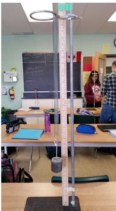
Figure 2: Experiment Apparatus Setup for Part 1 (Determining the Spring Constant)
