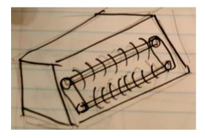
3. In this image, it shows the ball collector have in a long "spinal" figure in the back that is slanted upward. This is much like a conveyor belt system but instead of a rubber material running through the "spine" so that the debris would move upward, the power of the arms will forcefully push up the debris to the top.
