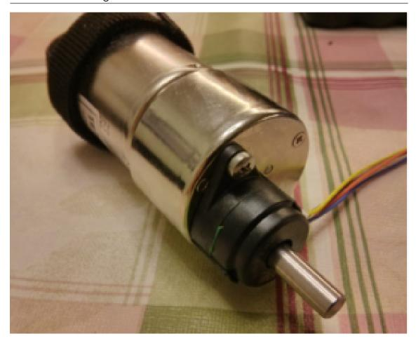
Figure 57.4: An encoder connected to a DC motor.
