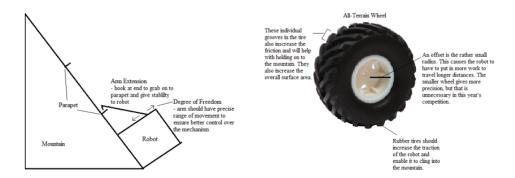
Figure 33.3: A diagram explaining the arm-like extension idea (left) and a diagram explaining the all-terrain wheel (right).
