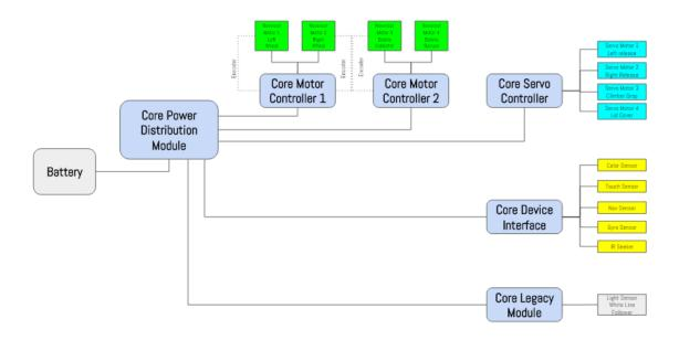
Figure 57.2: A more detailed diagram of the modules and other input and output functional parts.
