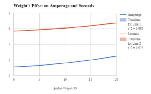
As seen from the data, the effect of weight on amperage and time needed for the robot to travel a distance of seven meters followed very strict exponential curves. Taking note of R-squared values of 0.992 and 0.973 for the best-fit lines, it can be con-
