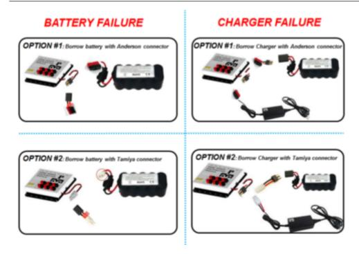
Figure 57.5: Chart depicting the steps needed to be taken in order to solve battery and charger failure.
