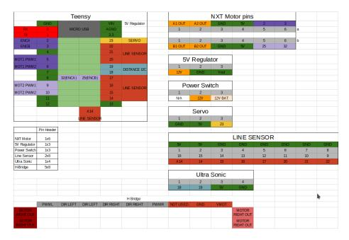
Figure 19: Pin Routing Specification Sheet
